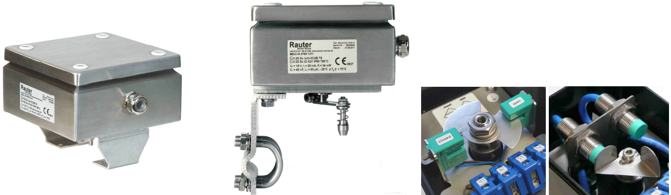
Pepperl+Fuchs limit switches: left: 2x adjustable aluminium switching cams. right: 1x stainless steel switching cam for position 0° and 90°. Other cams upon request.
