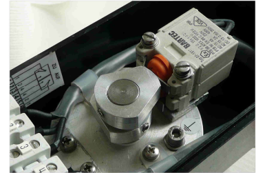
Bartec limit switches: 2x adjustable aluminium switching contacts
