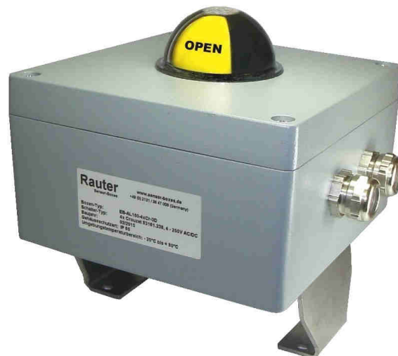
4 - 250 V AC/DC limit switch box with 3D indicator , aluminium housing, 160x160x90mm, 4x mechanical Crouzet switches SPDT, IP 65, - 20°C up to + 70°C
