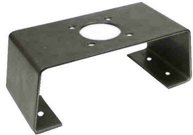
image.: brackets size 3 - 4 for actuators acc. to VDI/DE 3845, steam hight 30mm and 50mm, hole spacing 130x30mm
