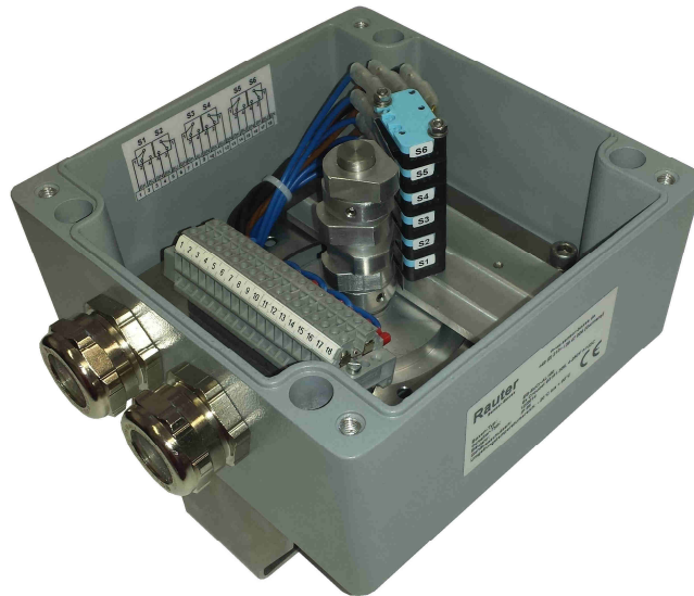
4 - 250 V AC/DC limit switch box security , aluminium housing, 160x160x90mm, 6x mechanical Crouzet switches SPDT , IP 65, - 20°C up to + 80°C
