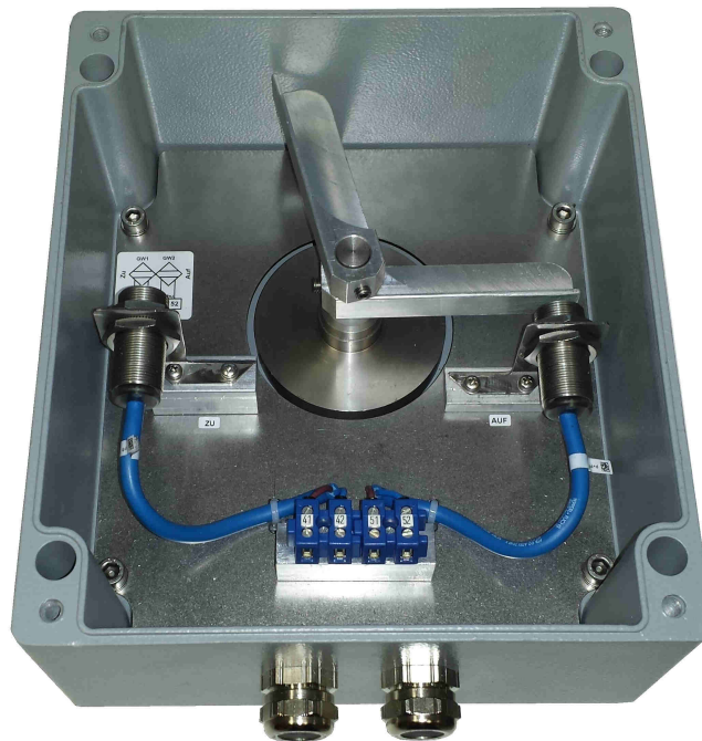
Ex i ... 8 V DC limit switch box hydraulic actuators with 75mm switch radius, aluminium housing, 230x200x110mm, 2x Pepperl+Fuchs sensor NCB5-18GM40-N0, IP 65, - 25°C up to + 70°C
