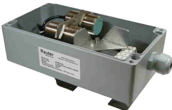
20 - 265 V AC/DC limit switch box , aluminium housing, 220x120x90mm, 2x Siemens-Bero sensors, IP 65, - 20°C up to + 60°C
