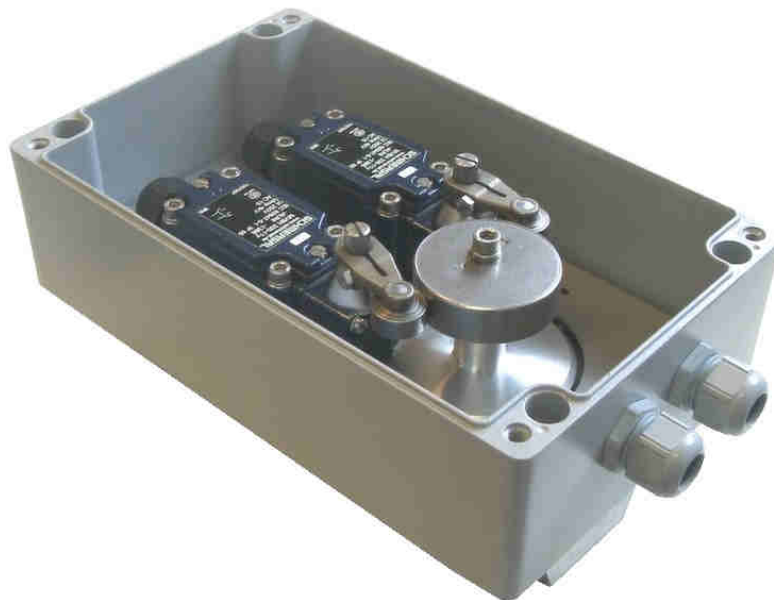
4 - 250 V AC/DC limit switch box , aluminium housing, 260x120x90mm, 2x mechanical Schmersal switches, IP 65, - 20°C up to + 60°C
