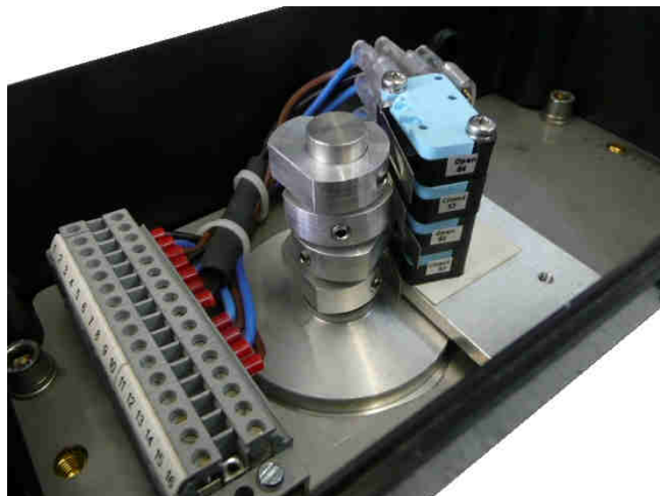
4 - 250 V AC/DC limit switch box , 6 mechanical Crouzet switches and 4x mechanical Crouzet switches, IP 65, - 20°C up to + 80°C
