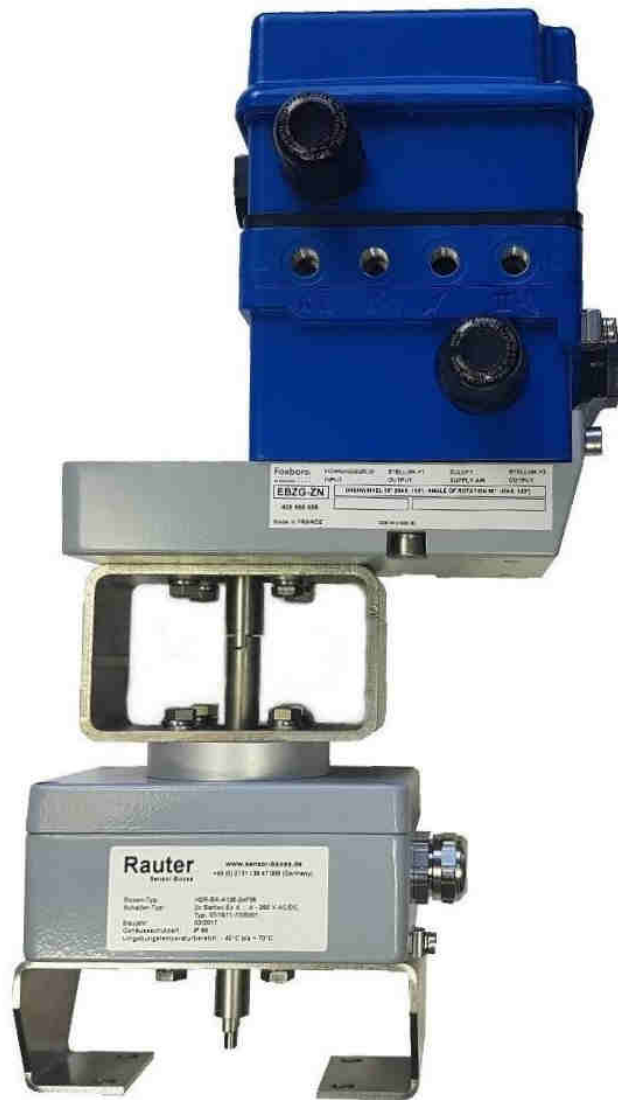
Ex ed ... 4 - 250 V AC/DC aluminium limit switch box, Abm.: 125x80x57, F05/F05-stainless steel bracket with Eckardt-Foxboro positioner and stainless steel bracket for actuators acc. to VDI/VDE 3845, Temperature range limit switch box: - 40°C up to + 70°C
