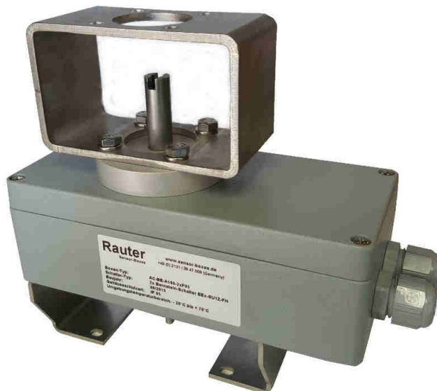
Image 6: Aluminium limit switch box, size: 175x80x57mm, Stainless steel bracket for actuators acc. to VDI/VDE 3845 and mounted stainless steel brackets F05/F05.
