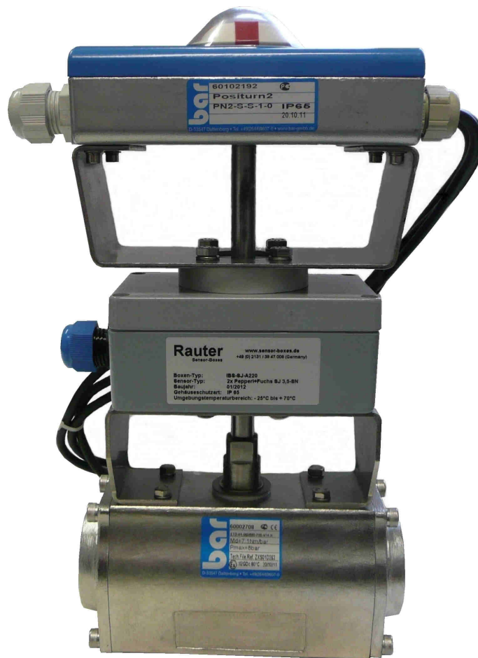
Image 2: Bar actuator with aluminium limit switch box, size: 125x80x57mm, stainless steel bracket for actuators acc. to VDI/VE 3845 and mounted Bar positioner
