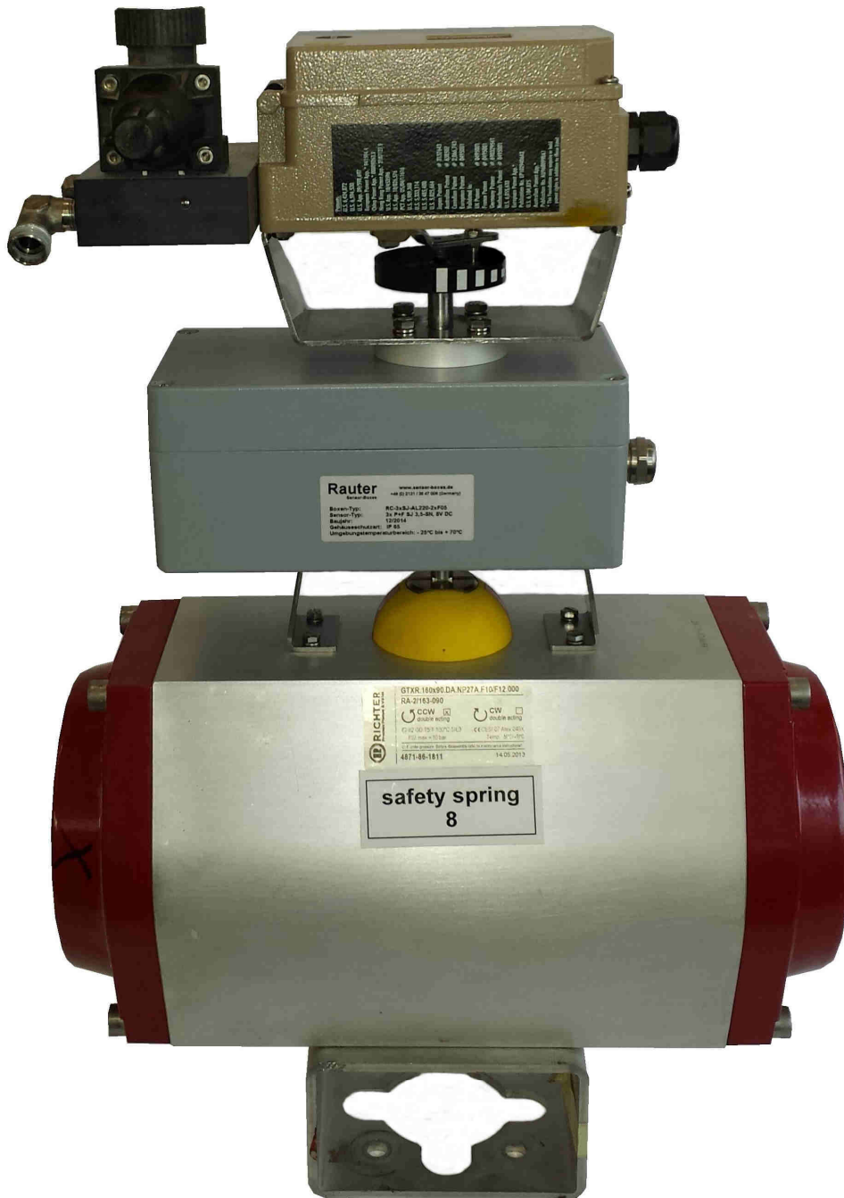
Image 3: Richter actuator with aluminium limit switch box, size: 220x120x90mm, stainless steel bracket for actuators acc. to VDI/VDE 3845 and mounted Samson positioner
