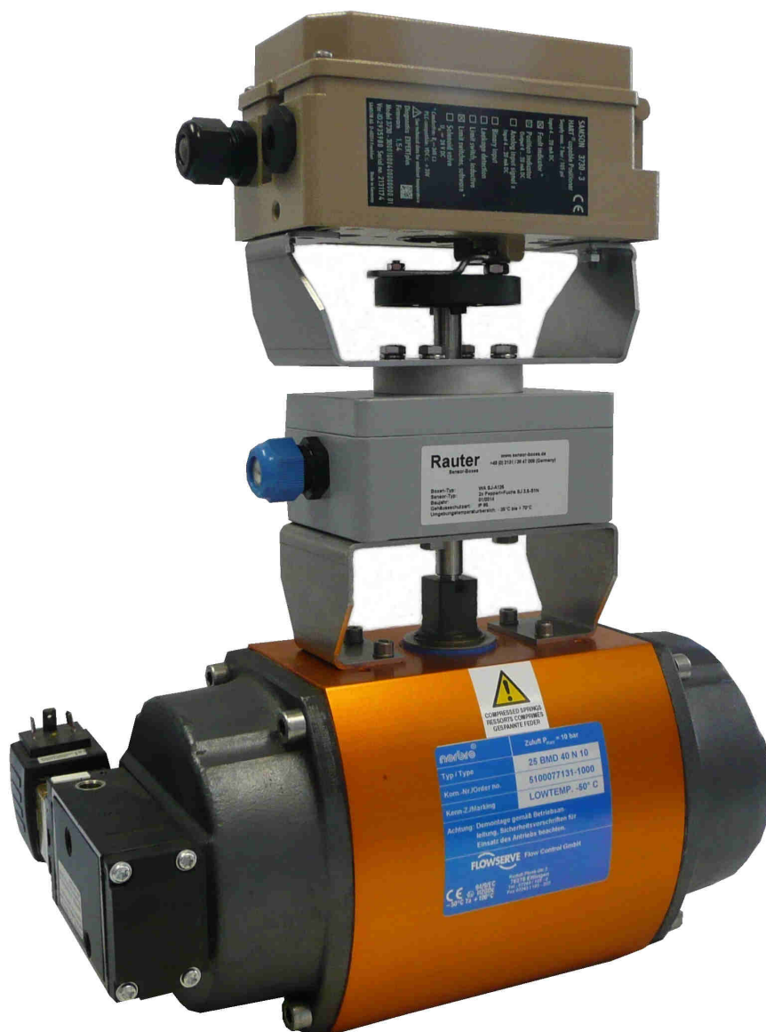
Image 1: Norbro actuator with aluminium limit switch box, size: 125x80x57mm, stainless steel bracket for actuators acc. to VDI/VDE 3845 and mounted Samson positioner.
