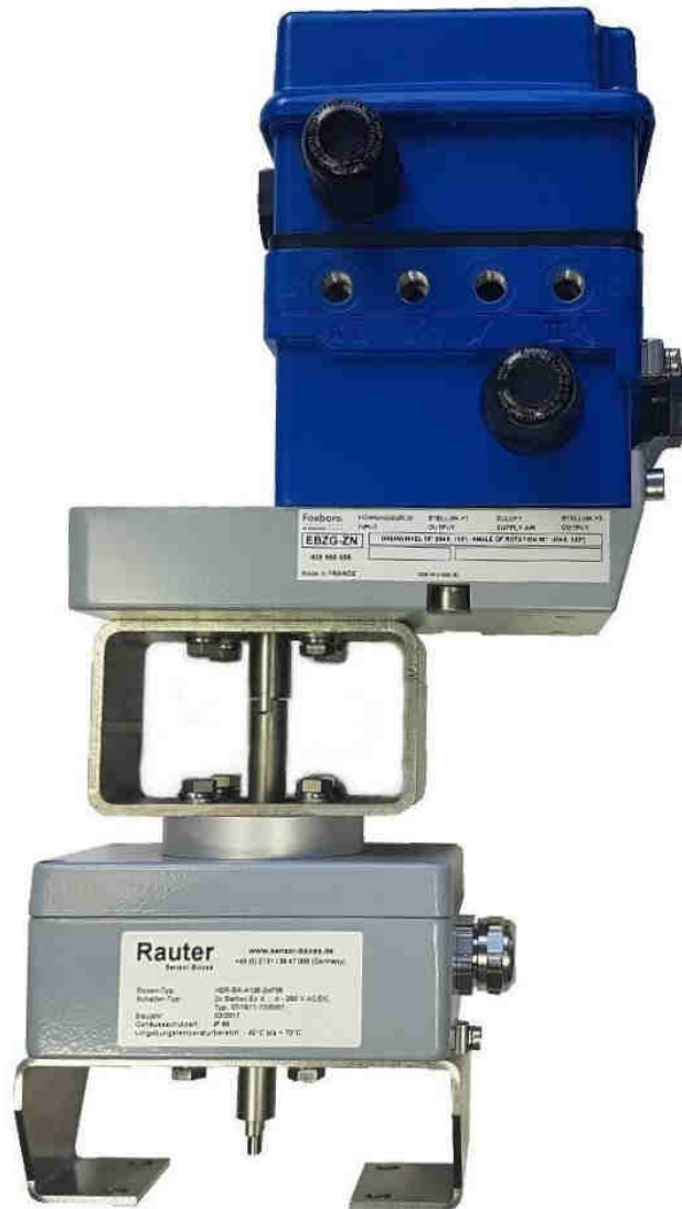
Image 4: Aluminium limit switch box, size: 125x80x57, F05/F05 stainless steel bracket with Eckardt-Foxboro positioner and stainless steel bracket for actuators with slot acc. to VDI/VDE 3845, temperature range limit switch box: - 40°C up to + 70°C
