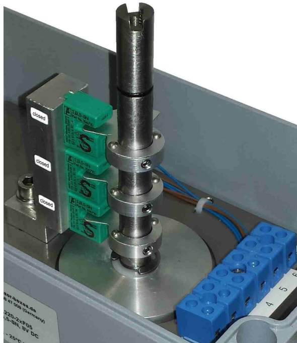
Image 8: 3x Pepperl+Fuchs sensors SJ 3,5-SN for position closed with adjustable aluminium switching cams (with hexagon socket screw M4 SW 2mm) further more 6-pole clamp and going through stainless steel shaft with 2 O-rings
