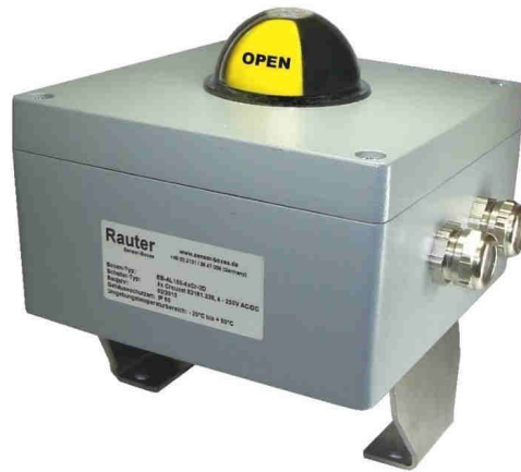
Image 4: 3D-aluminium limit switch box, 160x160x90mm for pneumatic actuators acc. to VDI/VDE 3845
