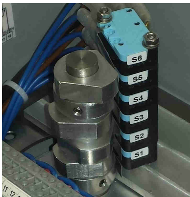
Image 1+2: left: 6x mechanical 4 - 250 V AC/DC Crouzet switches for any positions S1-S6 , right: 4x mechanical 4 - 250 V AC/DC Crouzet switches for any positions S1-S4
