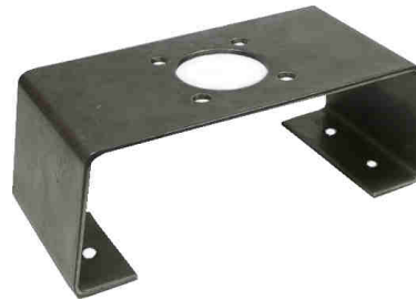
image.: brackets size 3 - 4 for actuators acc. to VDI/VDE 3845, steam high 30mm and 50mm, hole spacing 130x30mm
