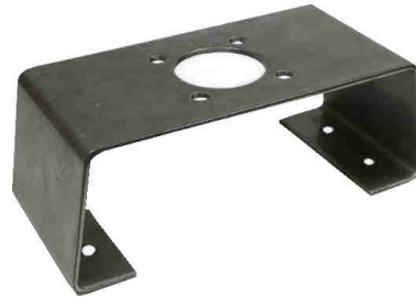
image.: brackets size 3 - 4 for actuators acc. to VDI/VDE 3845, steam high 30mm and 50mm, hole spacing 130x30mm
