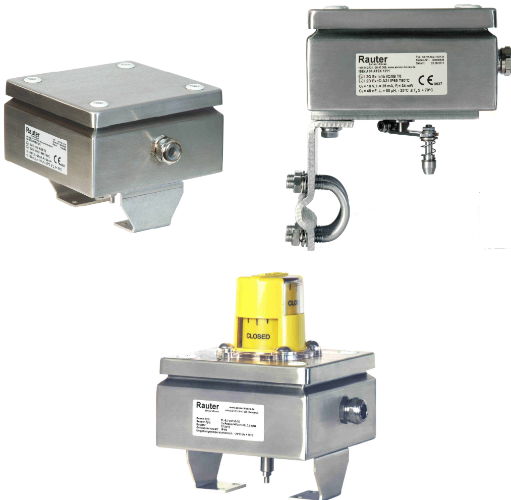
Image 1-3: left: stainless steel limit switch box, AISI 304, IP 65, 150x150x80 mm for rotary actuators acc. to VDI/VDE 3845 with bracket, right: with mounting set for linear actuators acc. to NAMUR IEC 534, below: with 3D indicator OPEN/CLOSED for rotary actuators with bracket
