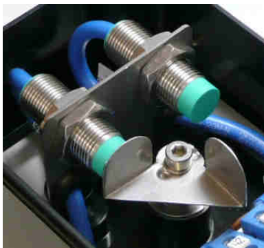
Image 6+7: left: 2x Pepperl+Fuchs sensors NJ2-12GK-N with stainless steel switching cam for position 0° and 90°, right: 2x Pepperl+Fuchs sensors SJ 3,5-S1N with 2x adjustable switching cams for position 0° and 90°, which is tightened with a hexagon key SW = 2 mm.
