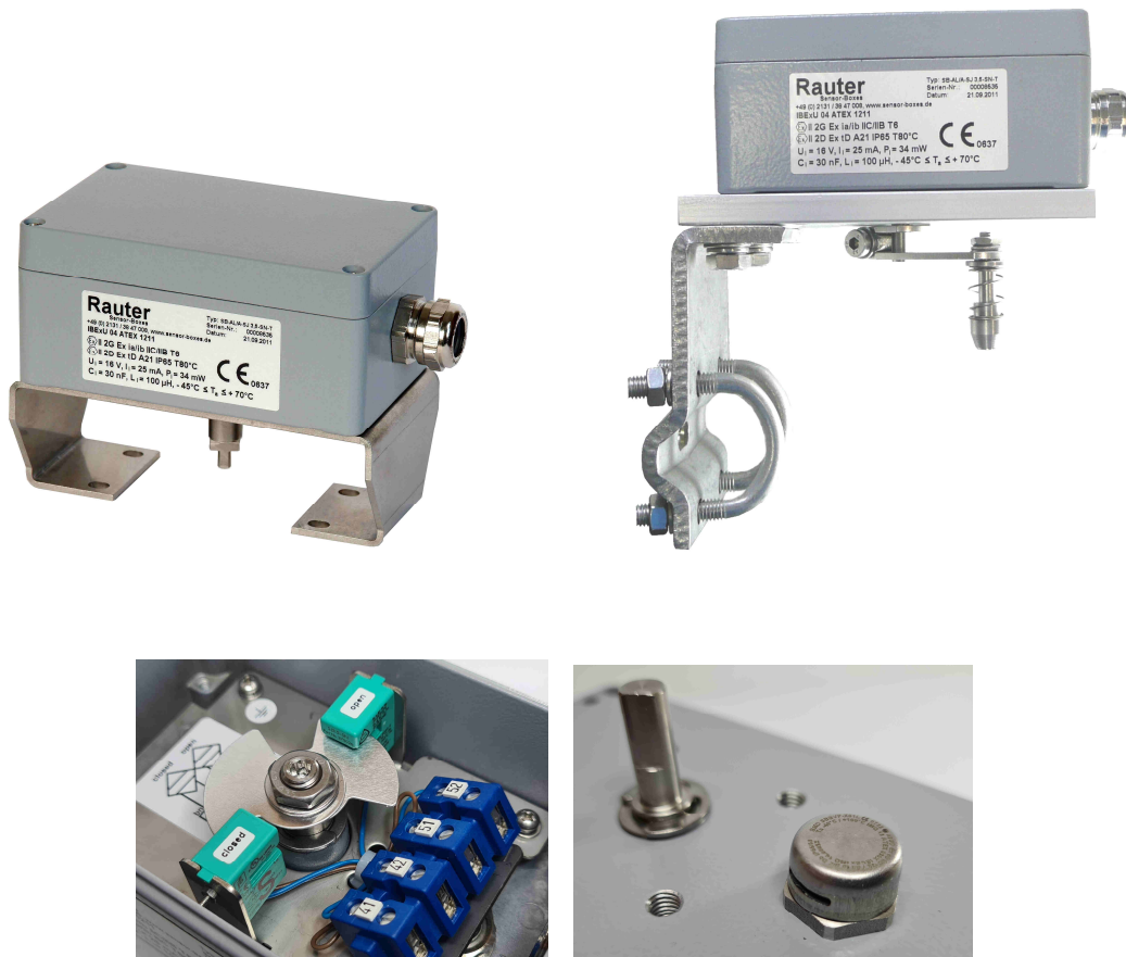
Images 1-4: Aluminium low temperature limit switch box, size.: 125x80x57 mm for rotary- and linear actuators with 2x Pepperl+Fuchs sensors SJ 3,5-SN, image 4: stainless steel membrane vent in limit switch box for linear actuator without aluminium plate.
