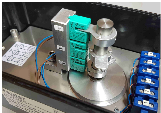
Image 11+12: 2x SJ 3,5-N for 2x position open, 3x SJ 3,5-N for position 0°, 120° and 240°
