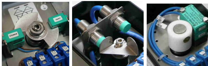
Image 24-26: inner views with P+F sensors SJ 3,5-SN (Image 24), NJ2-12GK-N (Image25), NJ2-V3 (Image 26)
