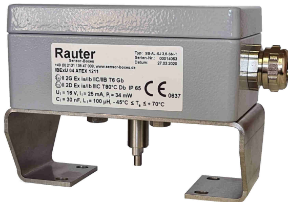
Image 20+21: Aluminium (125x80x57 mm) low temperature limit switch box with 2x Pepperl+Fuchs SJ 3,5-SN, ambient temperature range: -45\text{ °C} \leq T_a \leq +70\text{ °C}
