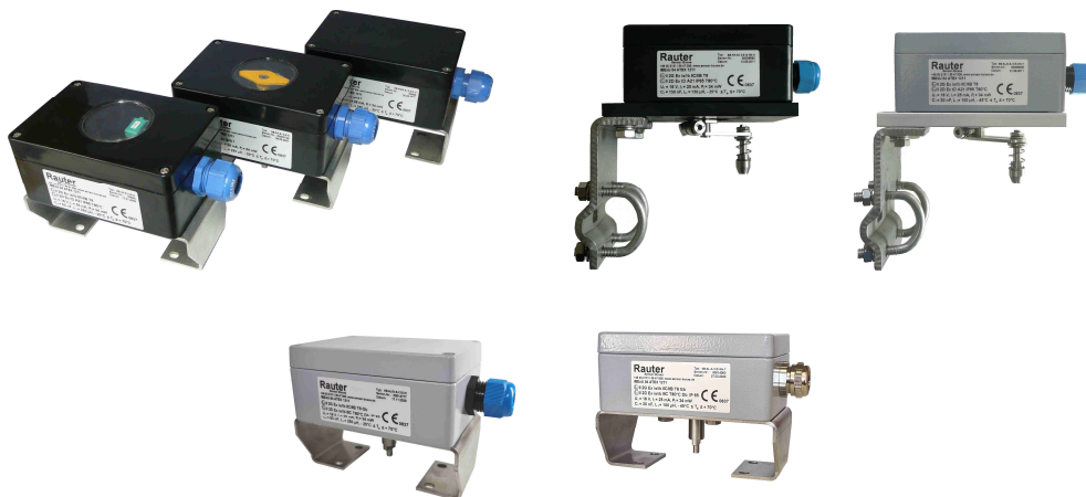
Image 1-4+4a: Image 1: polyamide limit switch boxes (this type with ex certification you can use specially in the mining industry), 120x80x55 mm for rotary actuators, Image 2+3: polyamide and aluminium limit switch boxes for linear actuators, 120/125x80x55/57 mm. Image 4 +4a: aluminium limit switch box and low temperature limit switch box for rotary actuators, 125x80x57 mm
