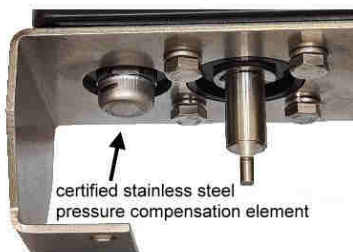
Image 27+27a+27b: Ex i ... 8 V DC polyamide limit switch box equipped with stainless steel membrane vent for avoidance of condensation water.
