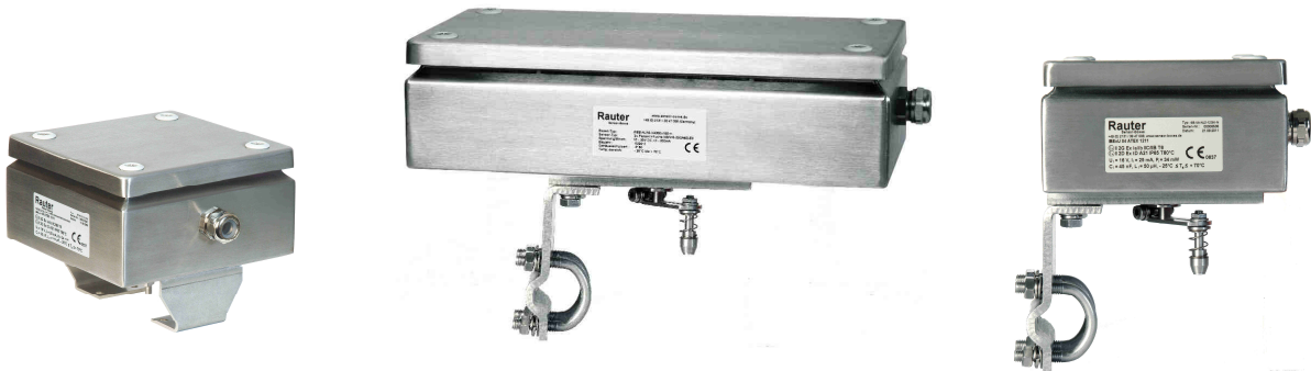
Image 1-3: left: stainless steel limit switch box, Aisi 304, size: 150x150x80mm, with stainless steel bracket for rotary actuators acc. to VDI/VDE 3845, middle and right: stainless steel limit switch box, Aisi 304, size: 300x150x80mm and size: 150x150x80mm with mounting set for linear actuators acc. to NAMUR IEC 534
