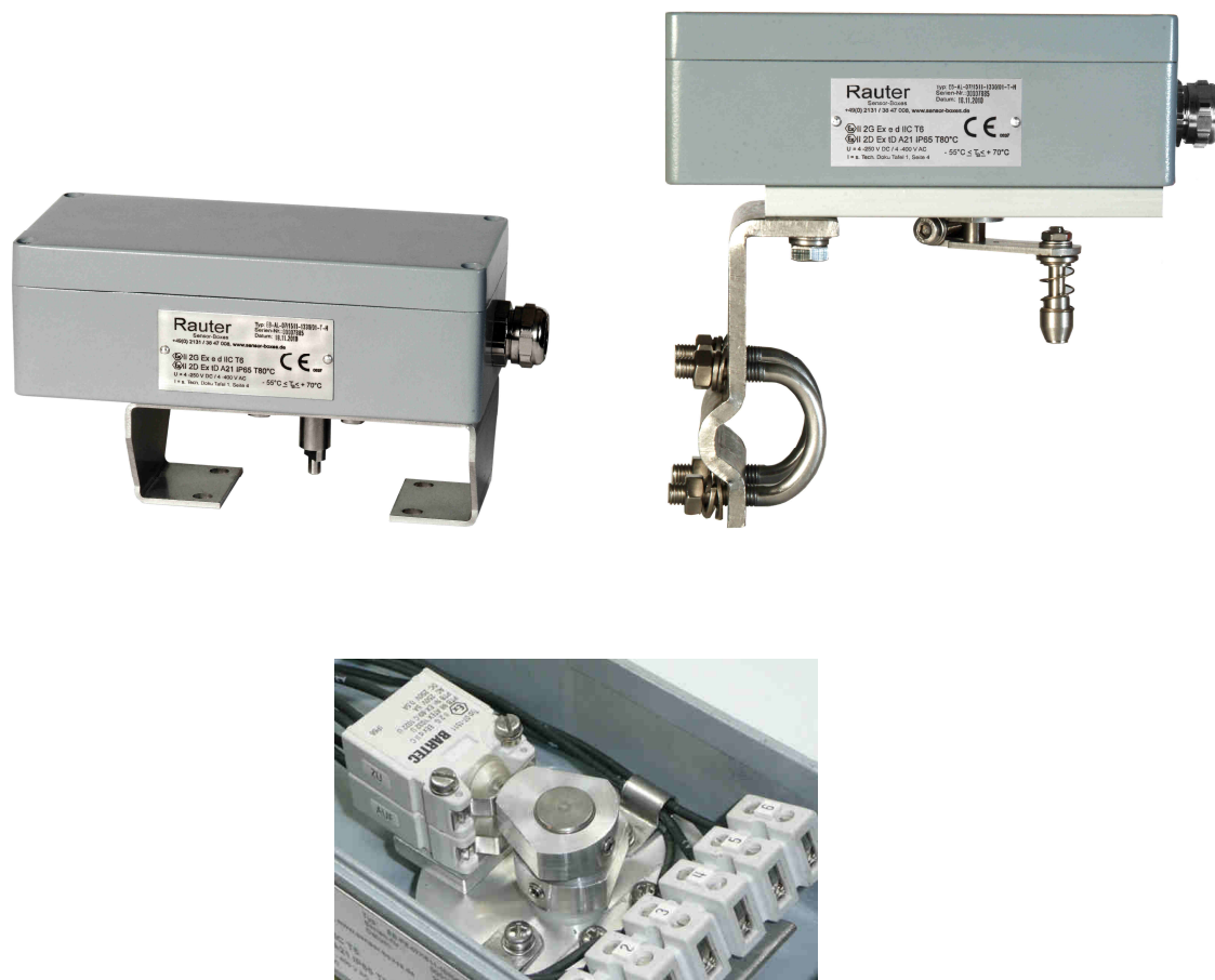
Image 1-3: Low temperature limit switch boxes with stainless steel bracket and stainless steel mounting set for rotary- and linear actuators, -55\text{ °C} \leq T_a \leq +70\text{ °C} , 175x80x57 mm, IP 65. Inner view with adjustable switching contacts.
