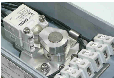
Image 12+13: Inner views low temperature limit switch boxes, -55^{\circ}\text{C} \leq T_a \leq +70^{\circ}\text{C} , with Ex d ... Bartec limit switches
