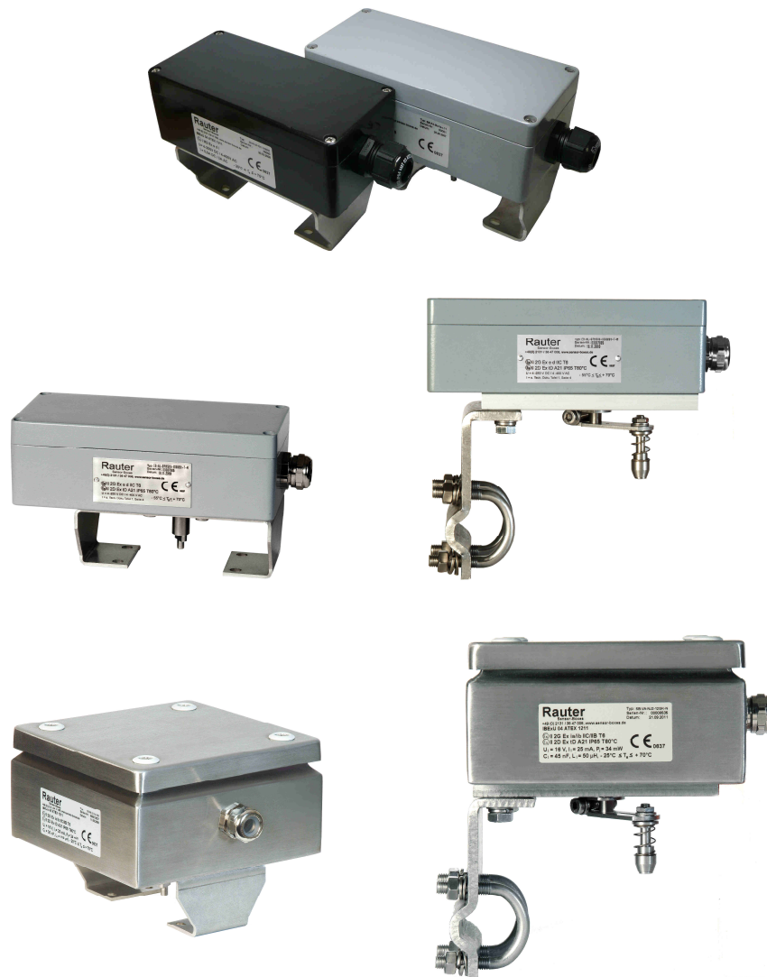
Image 1-5: Polyester- and aluminium limit switch boxes for rotary actuators, -20^{\circ}\text{C} \leq T_a \leq +70^{\circ}\text{C} , 160x75x55mm/175x80x57mm, IP 65, low temperature limit switch boxes for rotary and linear actuators, -55^{\circ}\text{C} \leq T_a \leq +70^{\circ}\text{C} , 175x80x57mm, IP 65. Stainless steel limit switch boxes for rotary and linear actuators -20^{\circ}\text{C} \leq T_a \leq +70^{\circ}\text{C} , 150x150x80mm, IP 65.
