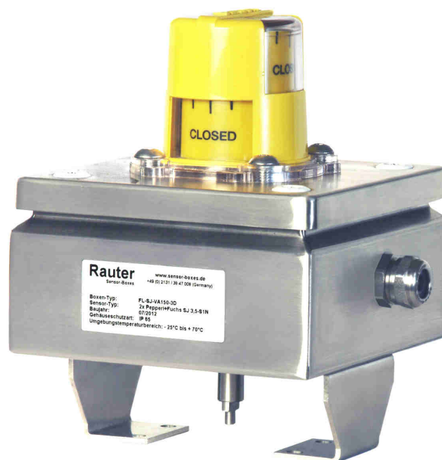
Image 1: stainless steel limit switch box, Aisi 304, with 3D-indicator, size.: 150x150x80mm, with stainless steel bracket, hole space 80x30mm for actuators acc. to VDI/VDE 3845 steam height 20mm
