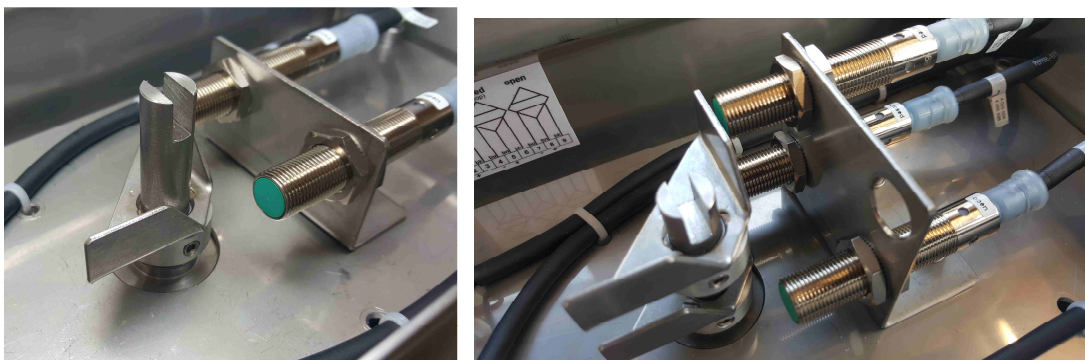
Image 2+3: Inductive Pepperl+Fuchs sensors NBB4-12GM45-E2-M for position (left) 1x OPEN and 1x CLOSED and (right) 1x OPEN and 2x CLOSED with stainless steel/aluminium switching cams connected on 6 and 9-pole clamp.
